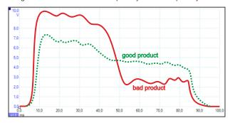
By visualizing the sensor signal, any defectives could be discovered which are caused by faulty weight distribtuion. It enables the operator to react immediately to machine or material irregularities.
